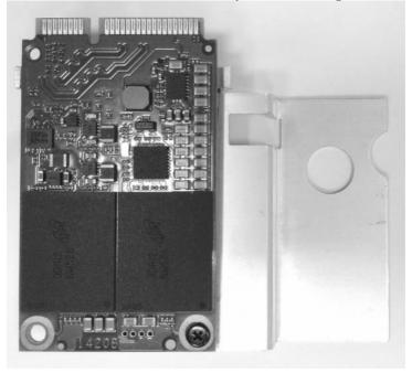
2. Install the mSATA with its heatplate into mSATA slot of the fitlet.
