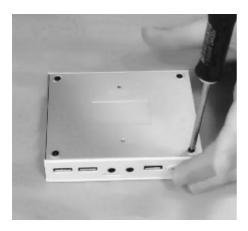
mSATA, SIM socket, miniPCIe and battery which are located at the bottom side of the motherboard are now accessible for installation/replacement.
