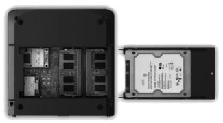
**Hard disk** is 2.5" 9.5mm SATA. It is screwed to service door by 4 screws, 2 on each side. It is recommended to use 5400 RPM hard disk or SSD. 7200 RPM or higher is not recommended due to their high power consumption and risk of overheating.
